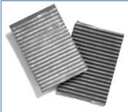
*HRC liners tend to resist moisture absorption, making it difficult to obtain a good bond.*
