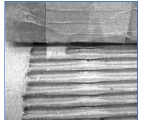
The problem appears to be caused by insufficient temperature and pressure. The tape needs to reach at least 215°F to melt the adhesive. Greater load pressure helps.
