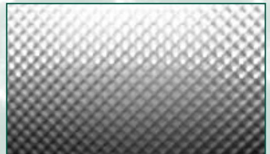
**After Calci-Kleen:** Closeup of glue roll. Full cell capacity is now available for adhesive.
