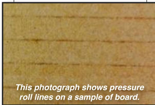
*This photograph shows pressure roll lines on a sample of board.*
