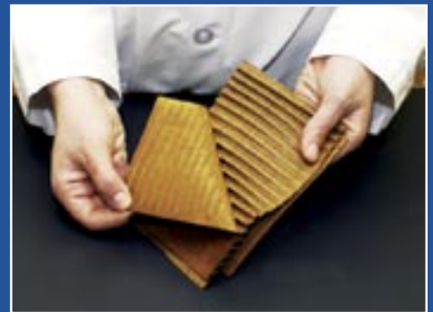
Lab technician checks the results of 24-Hour Soak Test, TAPPI T-812
