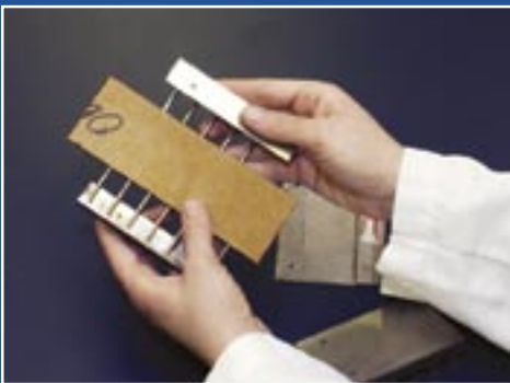
Lab technician prepares sample for wet-pin test, TAPPI T-821
