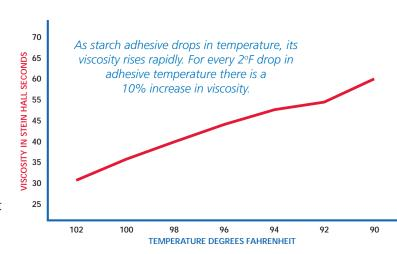
good working order to keep the adhesive at the proper temperature and viscosity. The TVC coils inside the tanks need to be free of starch build up that acts as an insulator. Insulating starch supply and return lines will help maintain adhesive temperature, especially in the extremely cold climates.
