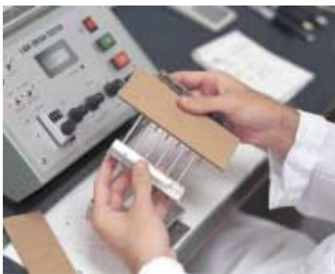
Dry pin adhesion test
