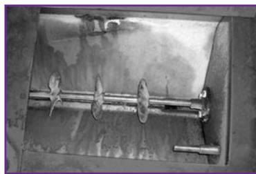
The secondary mixer (left) uses a set of marine type propellers to mix the cooked primary portion into the slurry. These tanks are usually rectangular in shape, with vee-shaped bottoms. A shaft runs horizontally across the bottom of the vee with two or three pairs of propellers mounted to it. Usually, each pair of propellers has opposite pitch so as to force the liquid into the end walls and generate more mixing force. Typically a motor of 10 HP to 20 HP drives the shaft via a vee-belt.
