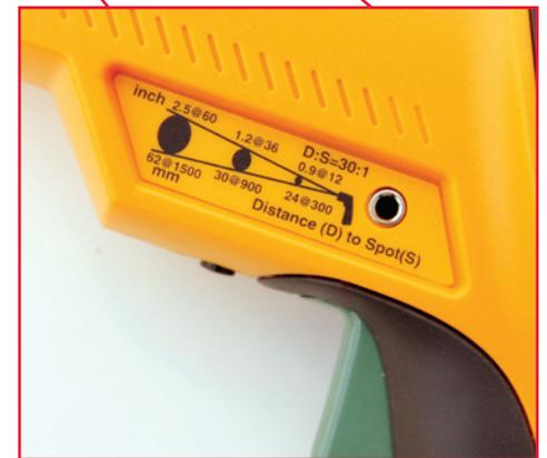
*IR heat guns usually have D:S ratio information printed or embossed for easy reference*
