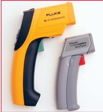
**H**andheld, noncontact infrared (IR) thermometers are widely used on the corrugator to measure paper and vessel temperatures. They allow for quick, safe measurements without physically touching either. These devices reveal an object's temperature by measuring the amount of infrared energy it is radiating.
