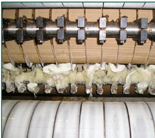
*Finger-type machines were often troubled by low gel-temperature adhesives gelling on the fingers.*
