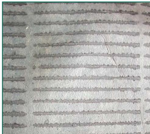
*Adhesive gelling on the fingers prevented starch from being applied in that area, creating finger blisters.*
