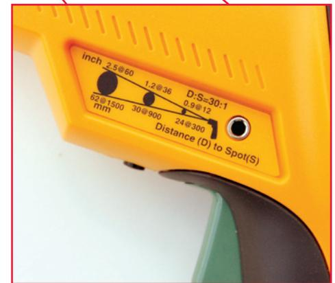
*IR heat guns usually have D:S ratio information printed or embossed for easy reference*
