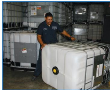
*When an empty tote is returned to our facility, it is inspected for serviceability. If the tote is determined to be serviceable, it is cleaned, repaired as needed, and tested to ensure fitness for use before being put back into service.*
