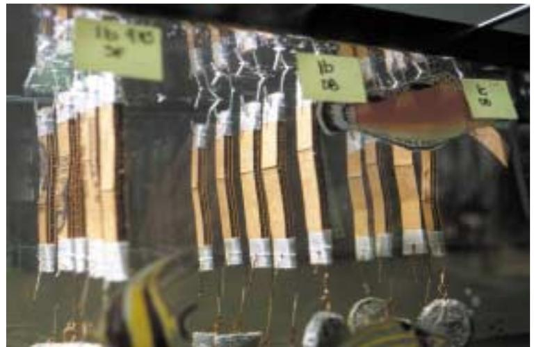
*In a recent demo, wet pin adhesion values improved by 62% (from 4.8 to 7.8 lbs/lineal feet) compared to a more standard-type adhesive, while the 24 hour soak produced 100% fiber tear.*
