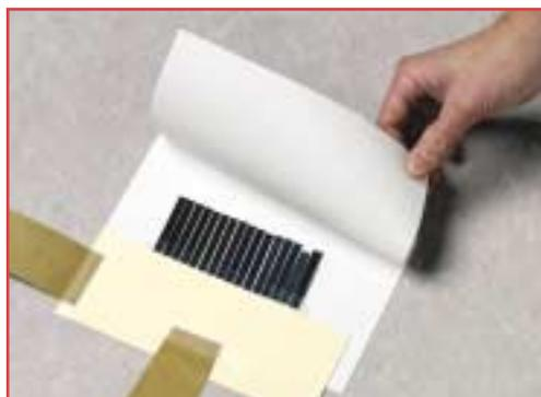
**4** To protect the strips until you are ready to use them, fold a letter-sized sheet of paper and tape it over the strips. The completed assembly can be stored with the flag and leader strip folded, and the protective sheet in place.
