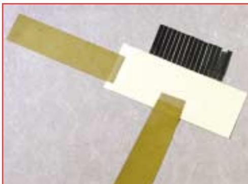
**3** Tape a short 8" flag extension onto the end of the assembly, and a long 24" leader strip to the center of the assembly. The 24" leader strip is necessary to keep hands away from the entrance nip.
