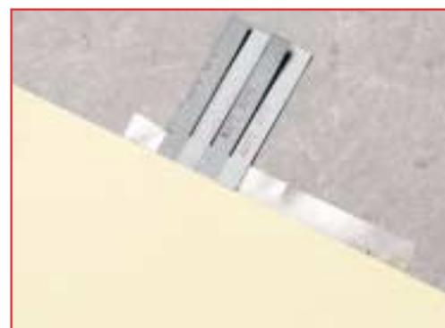
**1** Make an assembly of Thermopaper strips, ranging from 180°F to 340°F, in 10° increments.
