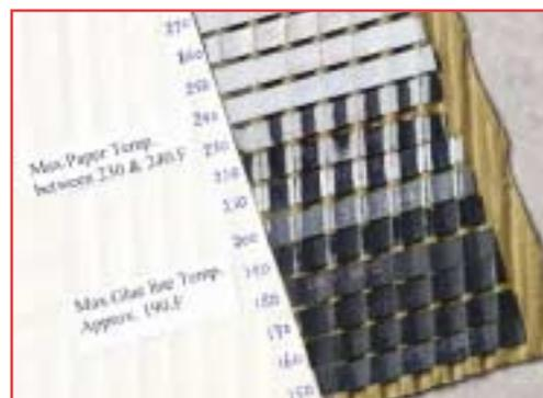
**6** Retrieve the marked sample from the stacker. The location of the assembly will be obvious because it causes a large blister. Cut the blister open to reveal the assembly, which will look similar to the photograph. The change in color will tell you the maximum temperatures of both the glue line and the liner.
