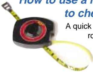
A quick and accurate way to check if two rolls are parallel to each other is to use a tape. If two rolls are parallel then the distance between them must be exactly the same at both ends and the middle.
