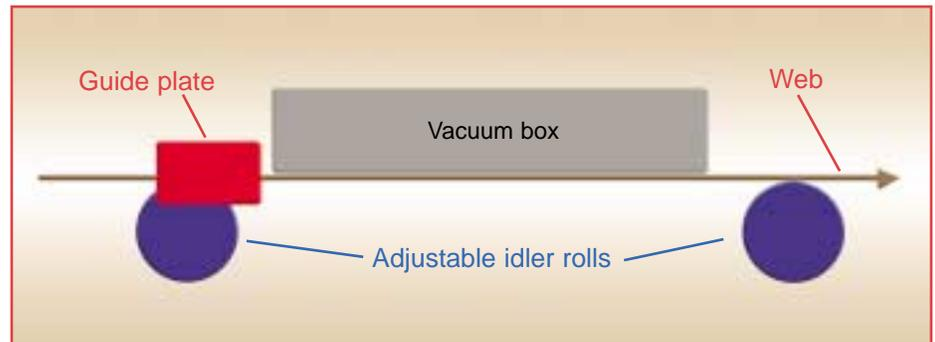
during width changes. When the double backer operator reduces or turns off the vacuum the web immediately moves to one side and contacts the guide plate. When the operator opens the side guides for the next paper width, the paper continues to walk off center, requiring corrective action.
