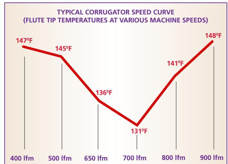
(as does bond quality). This is because, at very high speeds, the web spends very little time on the bridge, losing very little of its heat energy, therefore needing very little time on the preheater to replace lost energy. The accompanying graph demonstrates this phenomenon.
