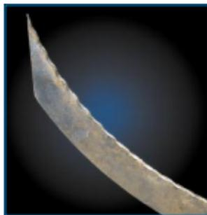
*Among other things, Bill Nikkel's update explores the problem of scalloped fingers. This wear pattern is a result of the finger vibrating against the paper-covered teeth. The contact that causes the wear also causes the pinching of the medium as it passes through this area. This pinching contributes to the development of high-low flutes.*
